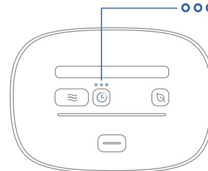
During the delay period, the **Cycle Delay** indicator lights above the button will illuminate **blue** until the Maintenance Cycle starts.
