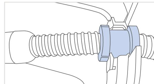
**C** Line up the Hose Sleeve with the gasket, place it in the Hose Slot and shut the lid.
