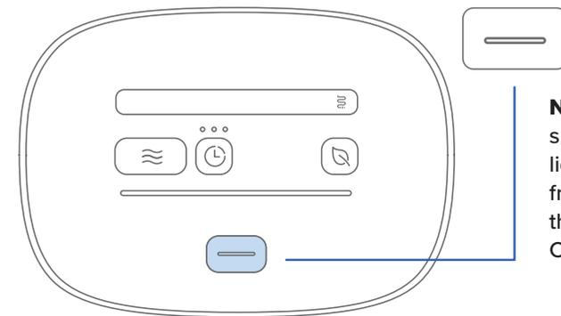
**NOTE:** The Lid will spring open and light will illuminate from the inside of the bottom of the Chamber.
