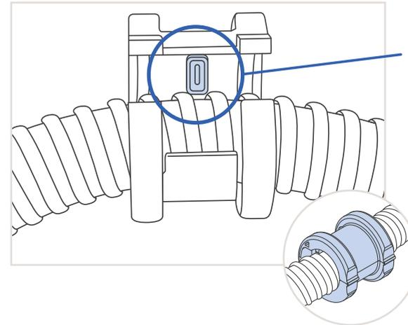
**B** Position the hose on the Nub side of the Hose Sleeve. Slide the hose until the Sleeve “clicks” into place between two of the hose ribs and close the Sleeve.
