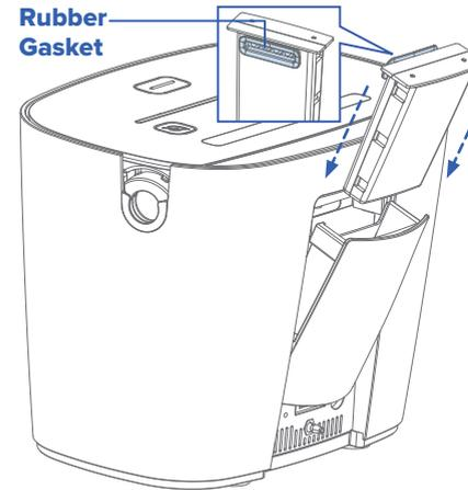
**C** Insert the **Filter** into the slot with the blue **Rubber Gasket** facing inward as shown.
