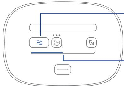
The **Progress Bar** on the Control Panel will illuminate **blue** from left to right as the cycle proceeds to completion.
