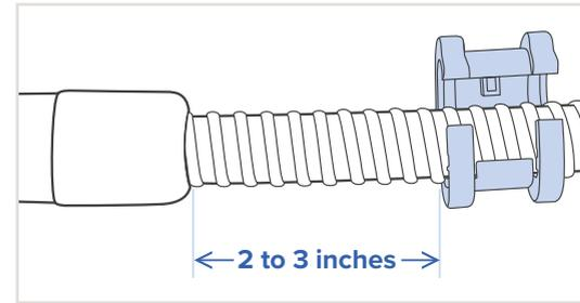
**A** Position the Hose Sleeve 2 to 3 inches from the connector.
