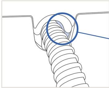
If there is visible space around the hose when placed in the hose slot, you may be using a 12 mm hose and require the Hose Sleeve be installed.
