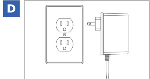
**D** Plug the **Power Supply** into an electrical outlet or power strip.
