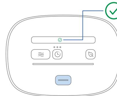
**C** At the end of the Cycle Delay and Maintenance Cycle, the **Cycle Complete** icon
